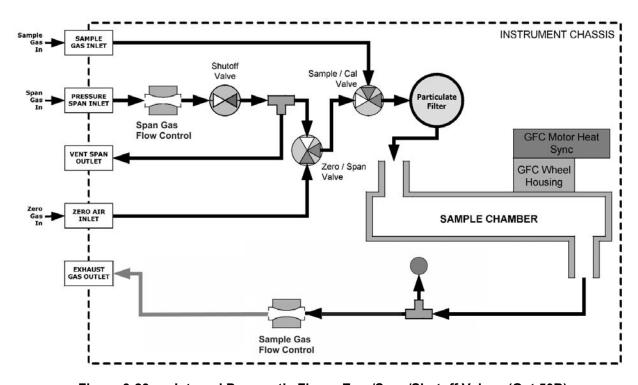
Figure 3-23: Internal Pneumatic Flow – Zero/Span/Shutoff Valves (Opt 50B)
